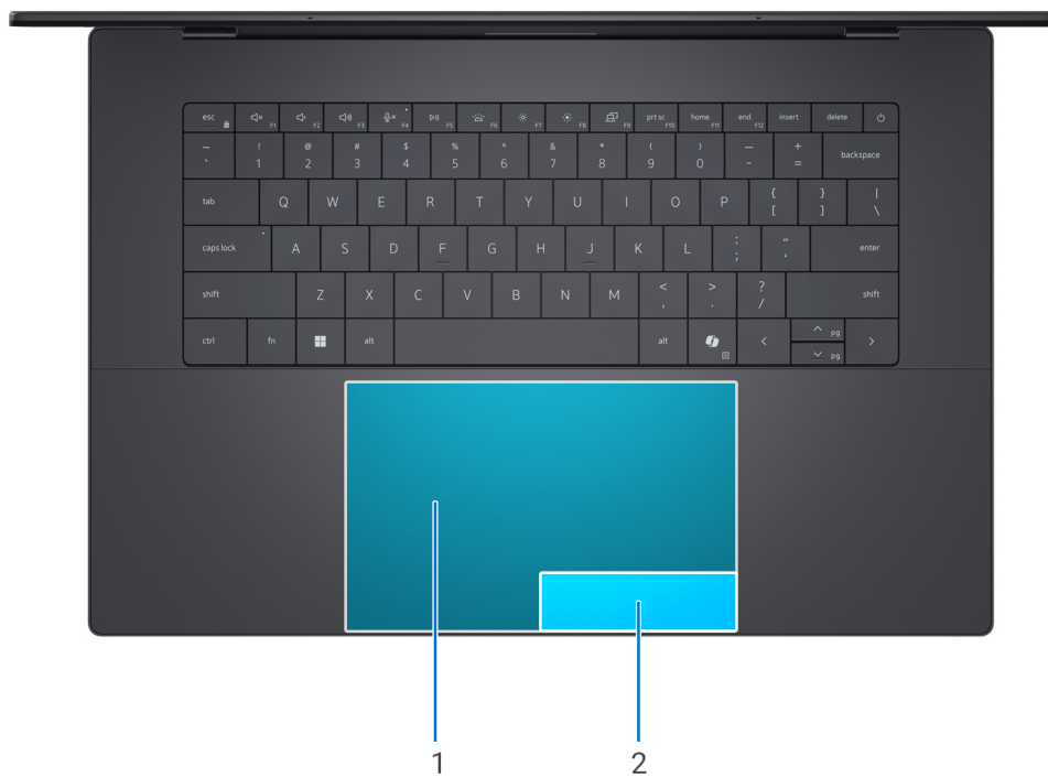
Figure 8. Active areas of the seamless touchpad
