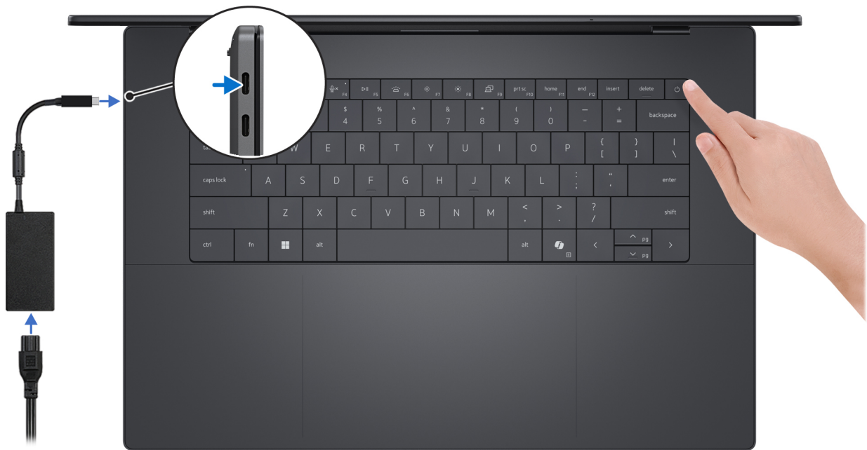
Figure 7. Connect the power adapter to the computer and power source, then press the power button to turn it on.
