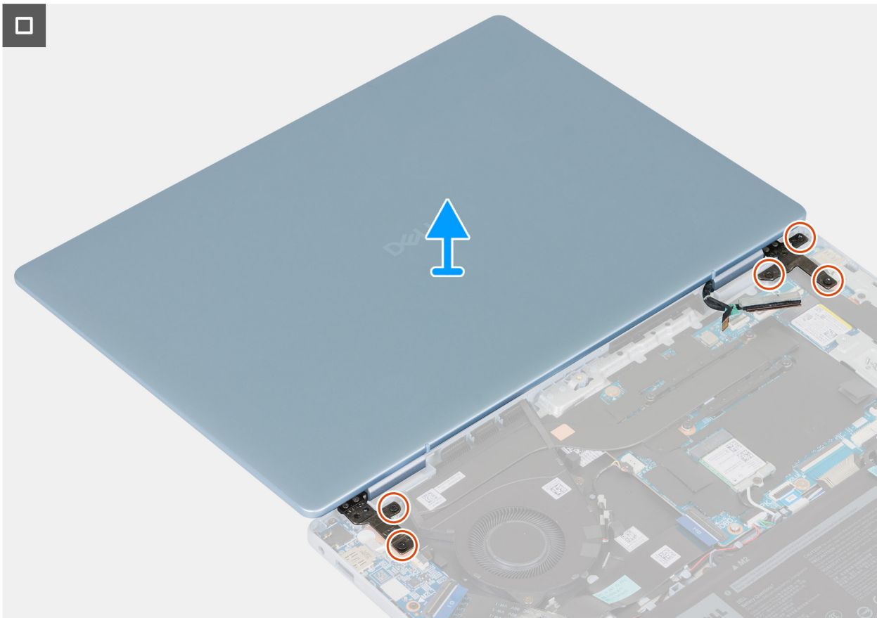
Figure 27. Removing the display assembly 2
