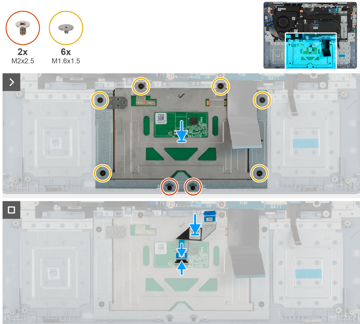
Figure 54. Installing the touchpad
