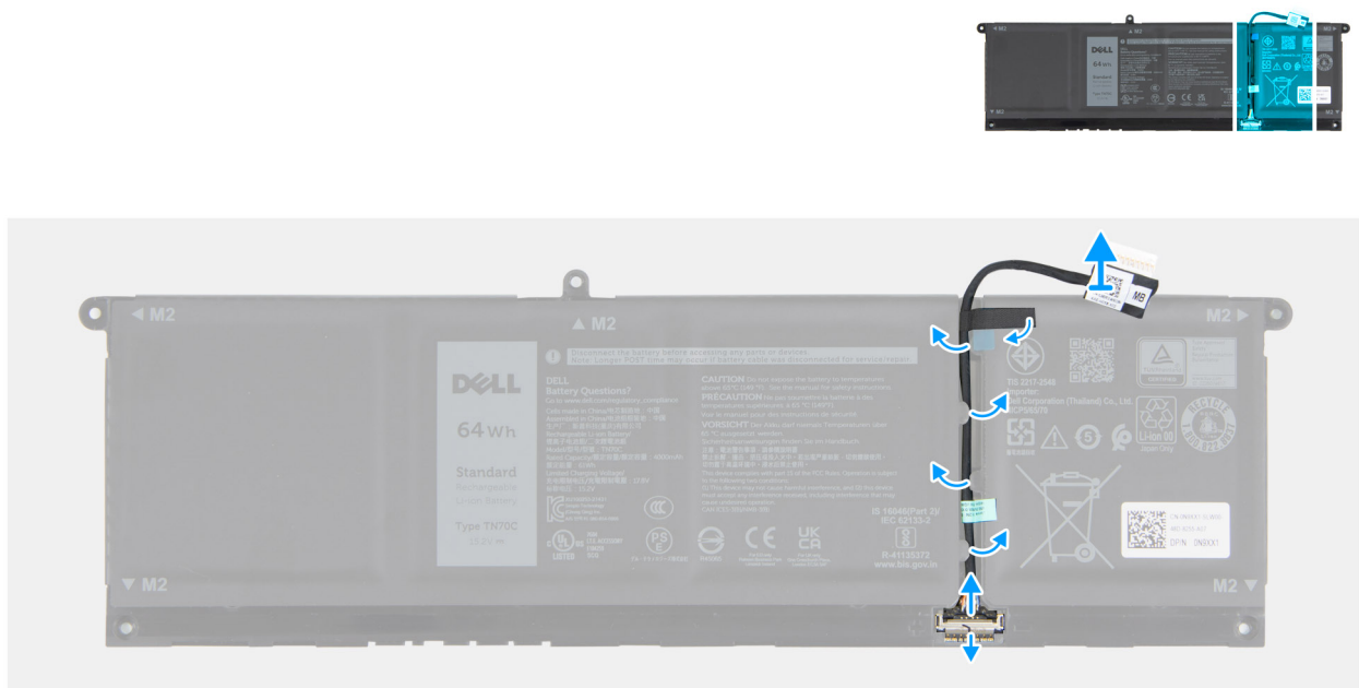
Figure 18. Removing the battery cable
