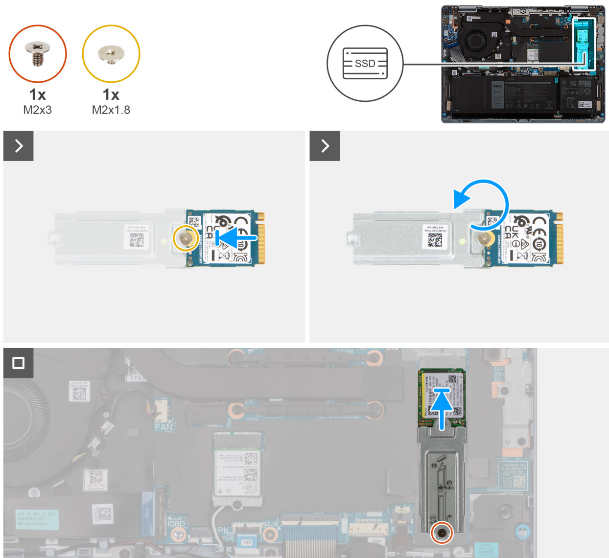
Figure 21. Installing the M.2 2230 solid state drive
