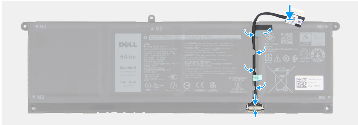
Figure 19. Installing the battery cable
