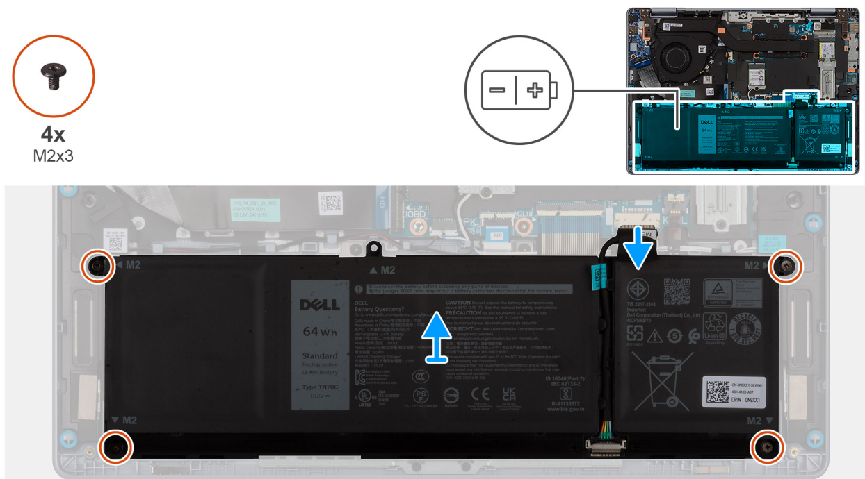
Figure 16. Removing the battery
