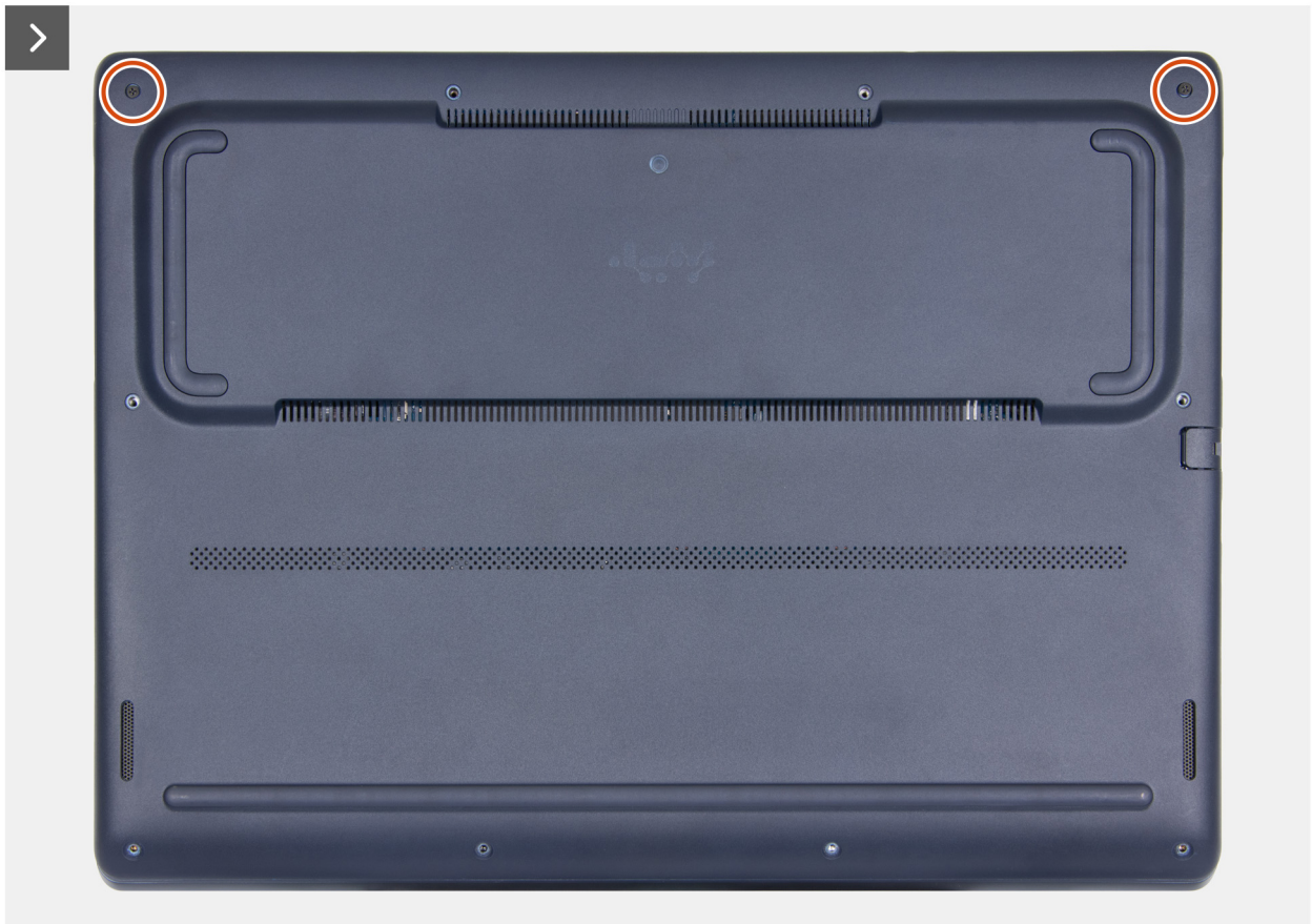
Figure 12. Loosening the captive screws on the base cover
