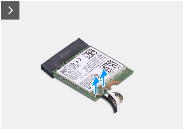
Figure 34. Removing the wireless card
