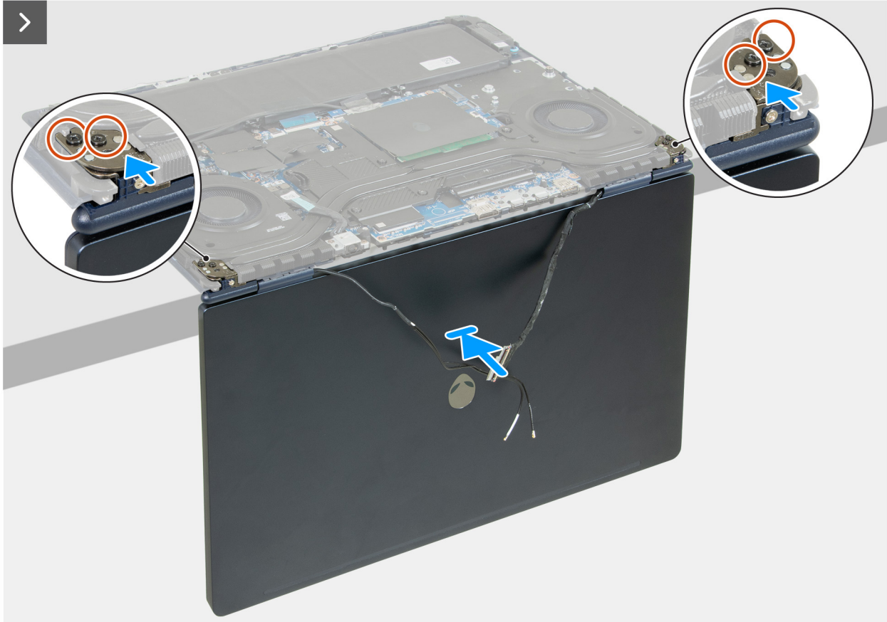
Figure 70. Installing the display assembly
