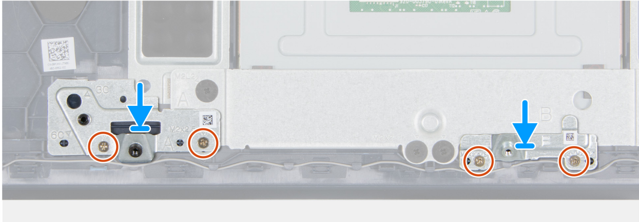
Figure 47. Installing the 6-cell battery brackets
