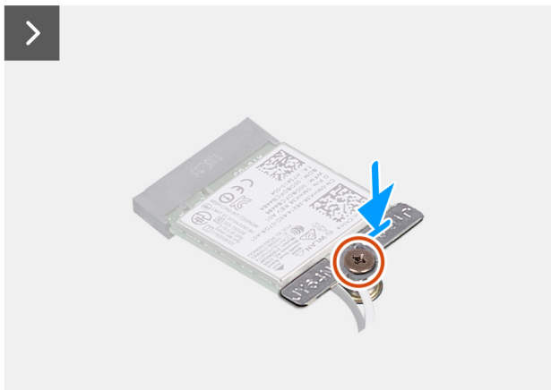
Figure 35. Installing the wireless card
