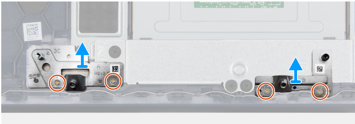
Figure 44. Removing the 3-cell battery brackets
