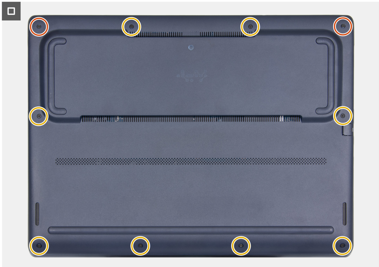
Figure 19. Installing the base cover
