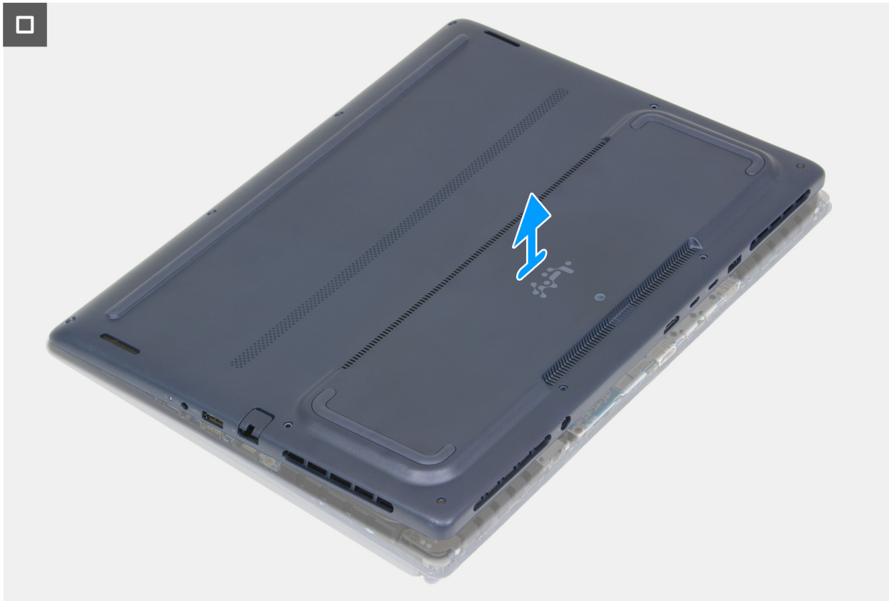
Figure 14. Removing the base cover
