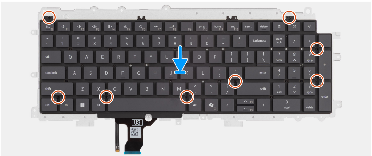
Figure 59. Installing the keyboard support plate
