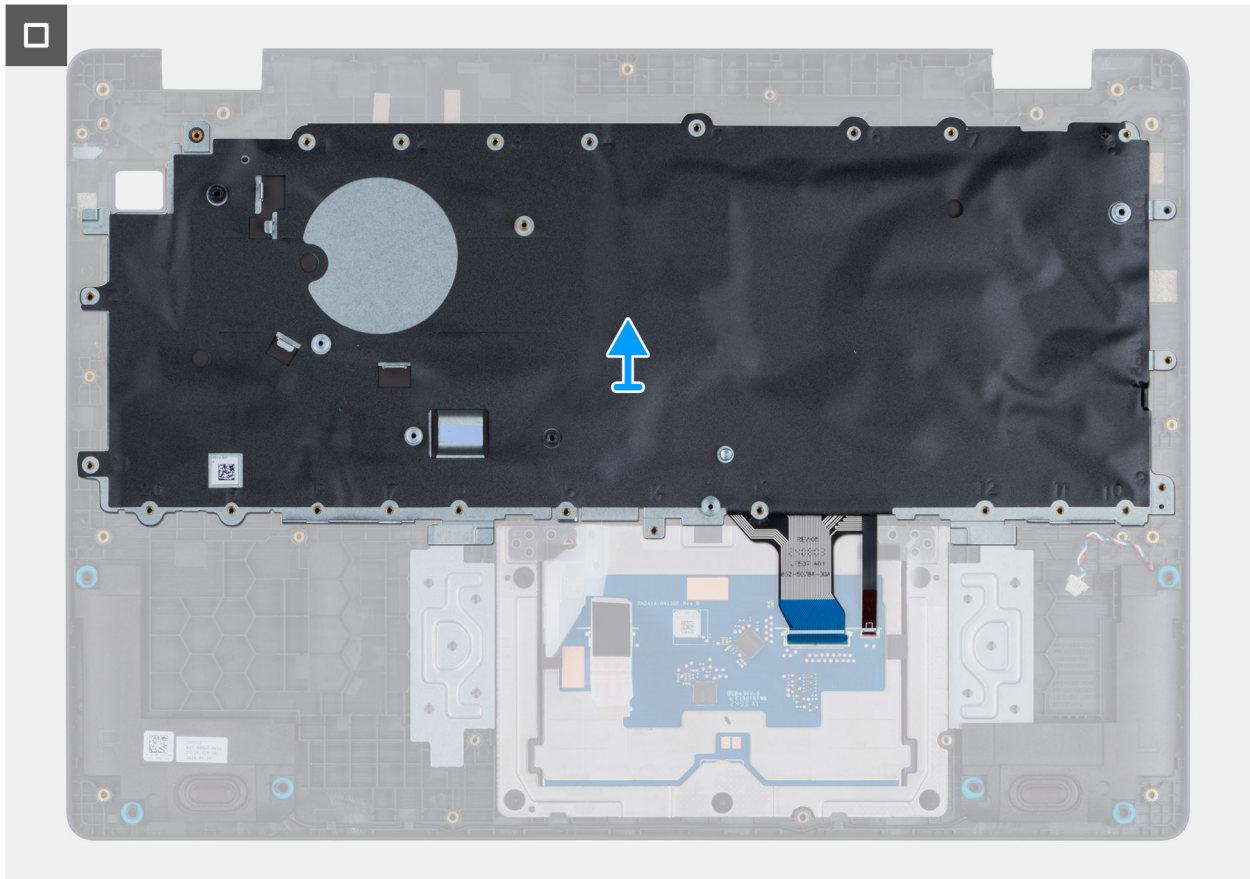
Figure 51. Removing the keyboard
