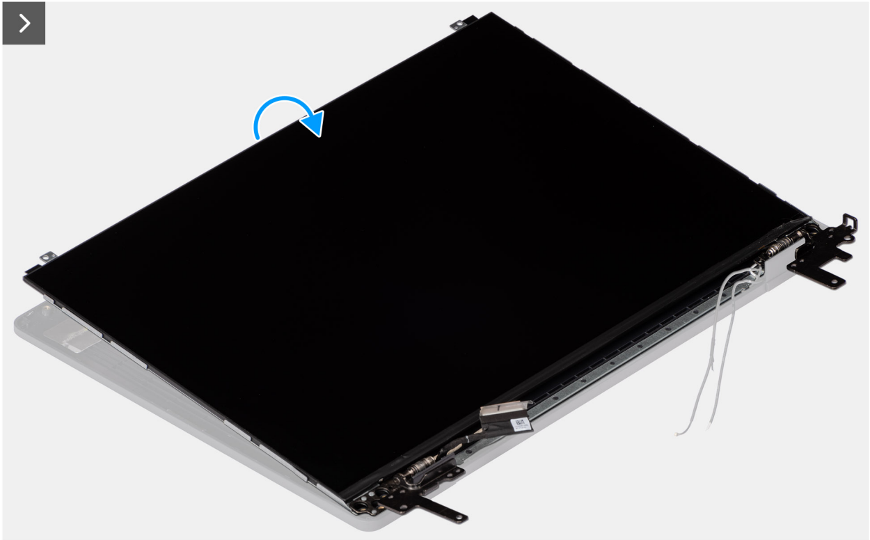
Figure 75. Removing the display-panel assembly
