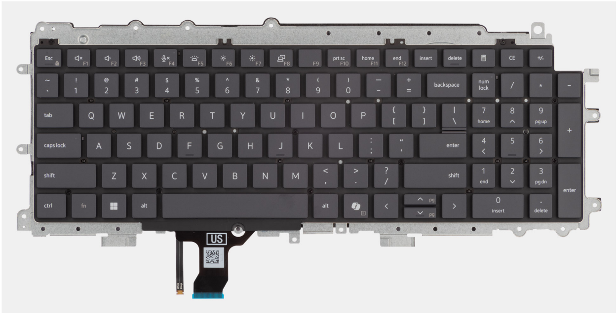
Figure 53. Installing the keyboard
