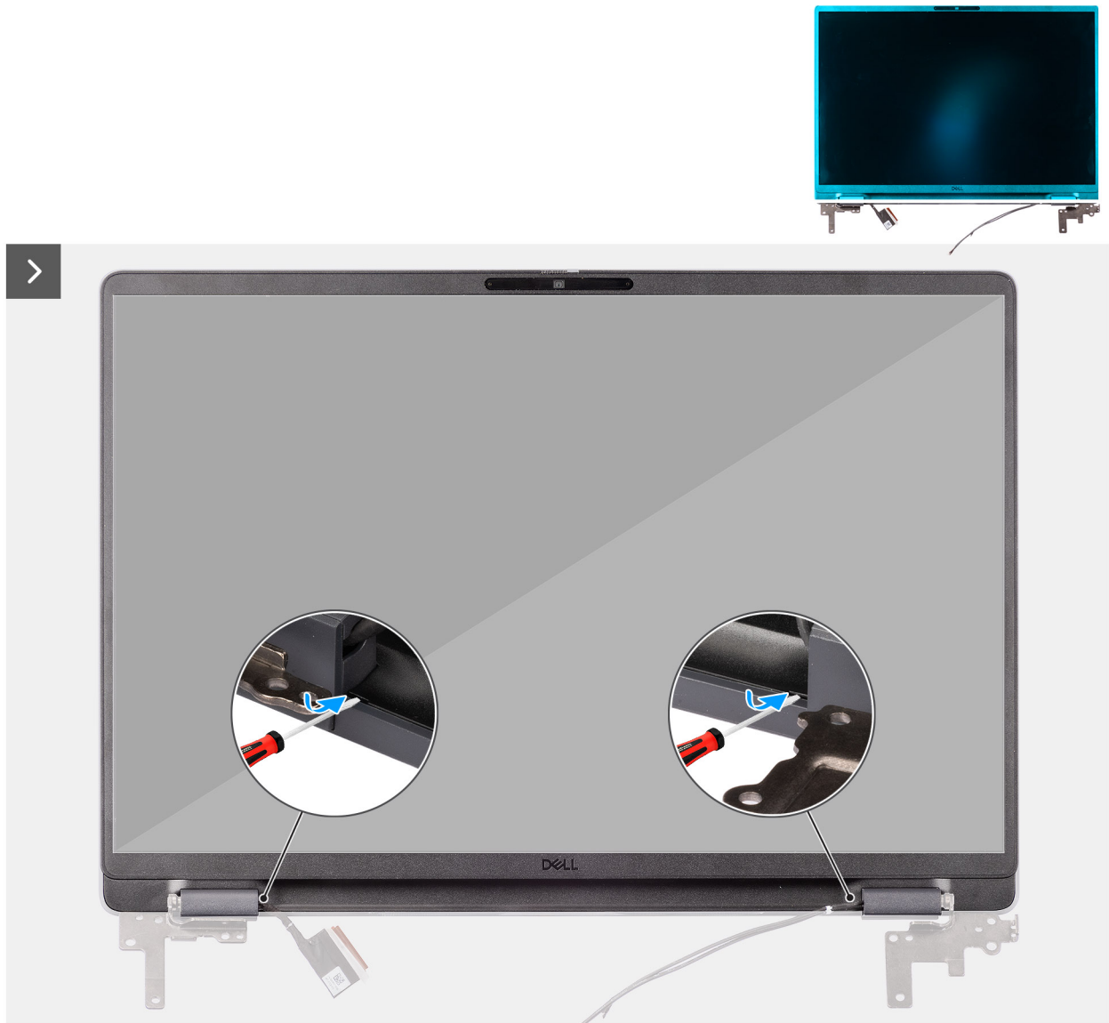
Figure 67. Removing the display bezel
