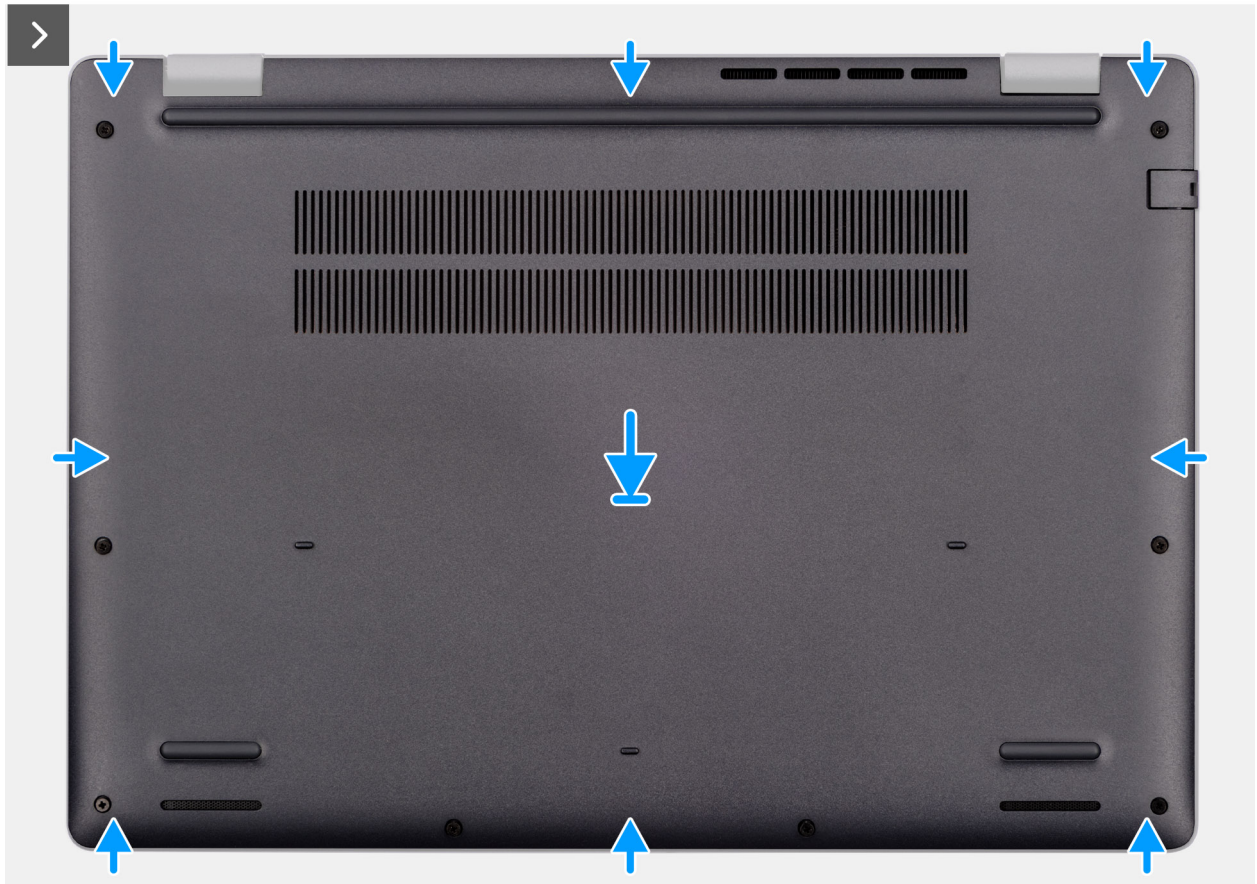
Figure 15. Installing the base cover
