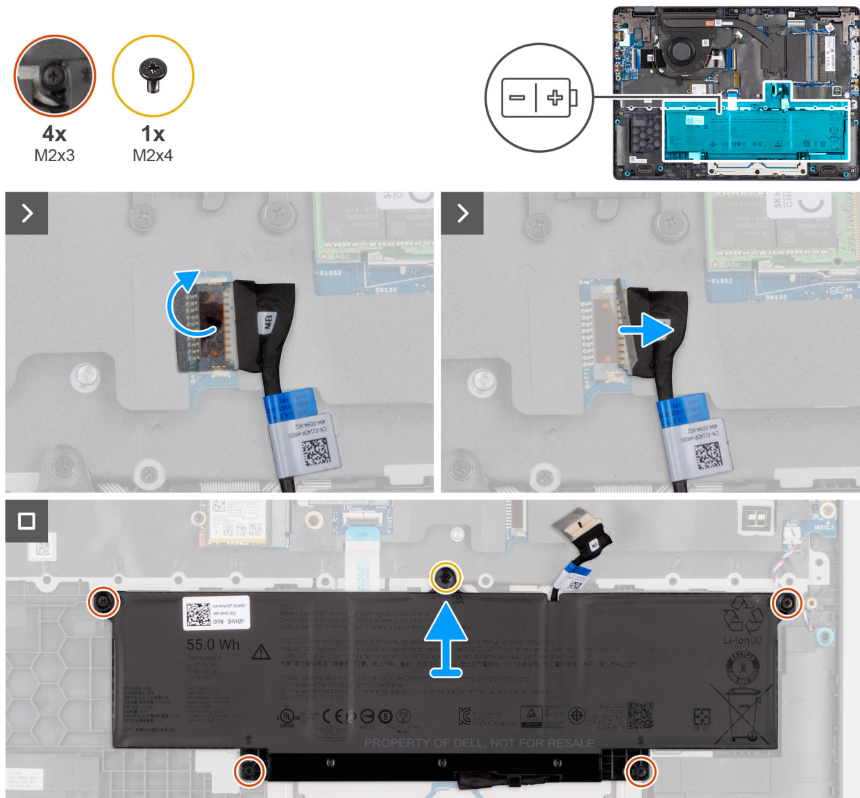
Figure 17. Removing the battery
