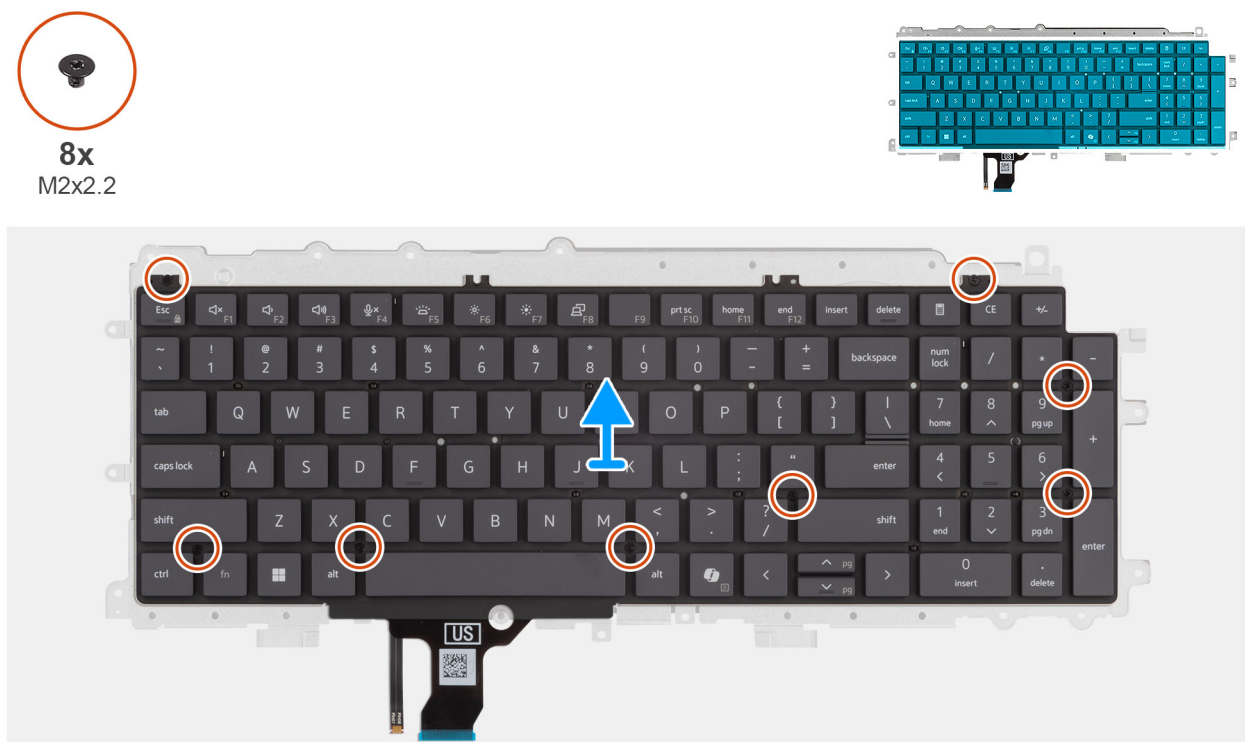
Figure 56. Removing the keyboard support plate
