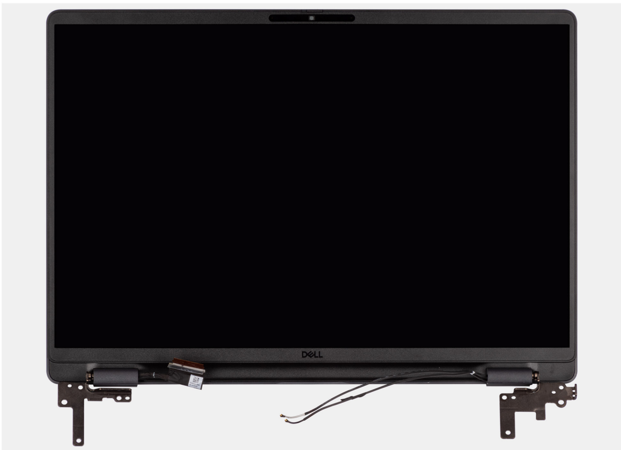
Figure 64. Removing the display assembly
