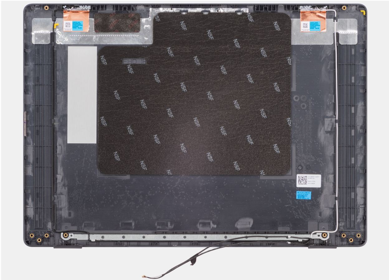
Figure 86. Removing the display back-cover assembly
