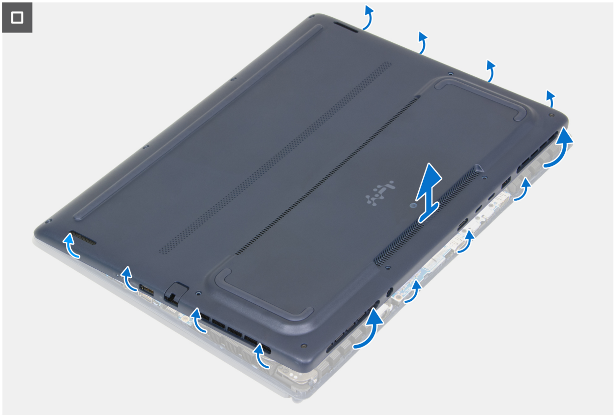
Figure 12. Removing the base cover
