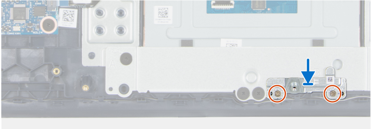
Figure 43. Installing the battery bracket
