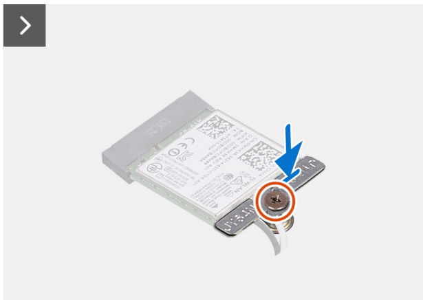
Figure 35. Installing the wireless card
