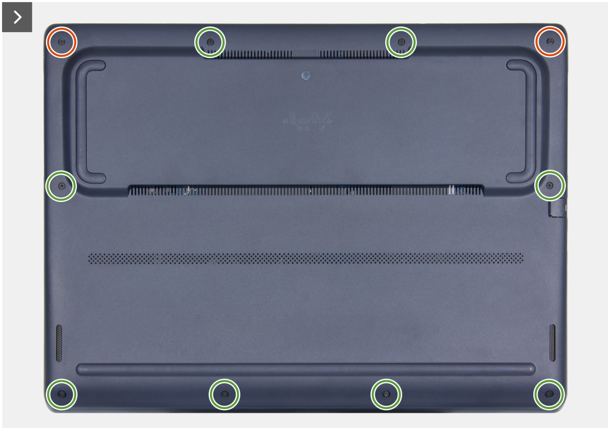
Figure 10. Removing the eight screws on the base cover
