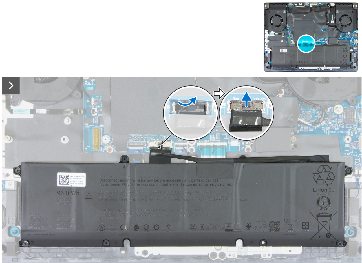
Figure 13. Disconnecting the battery cable
