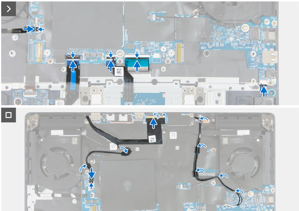
Figure 71. Installing the system board (for computers with VR heat sinks)
