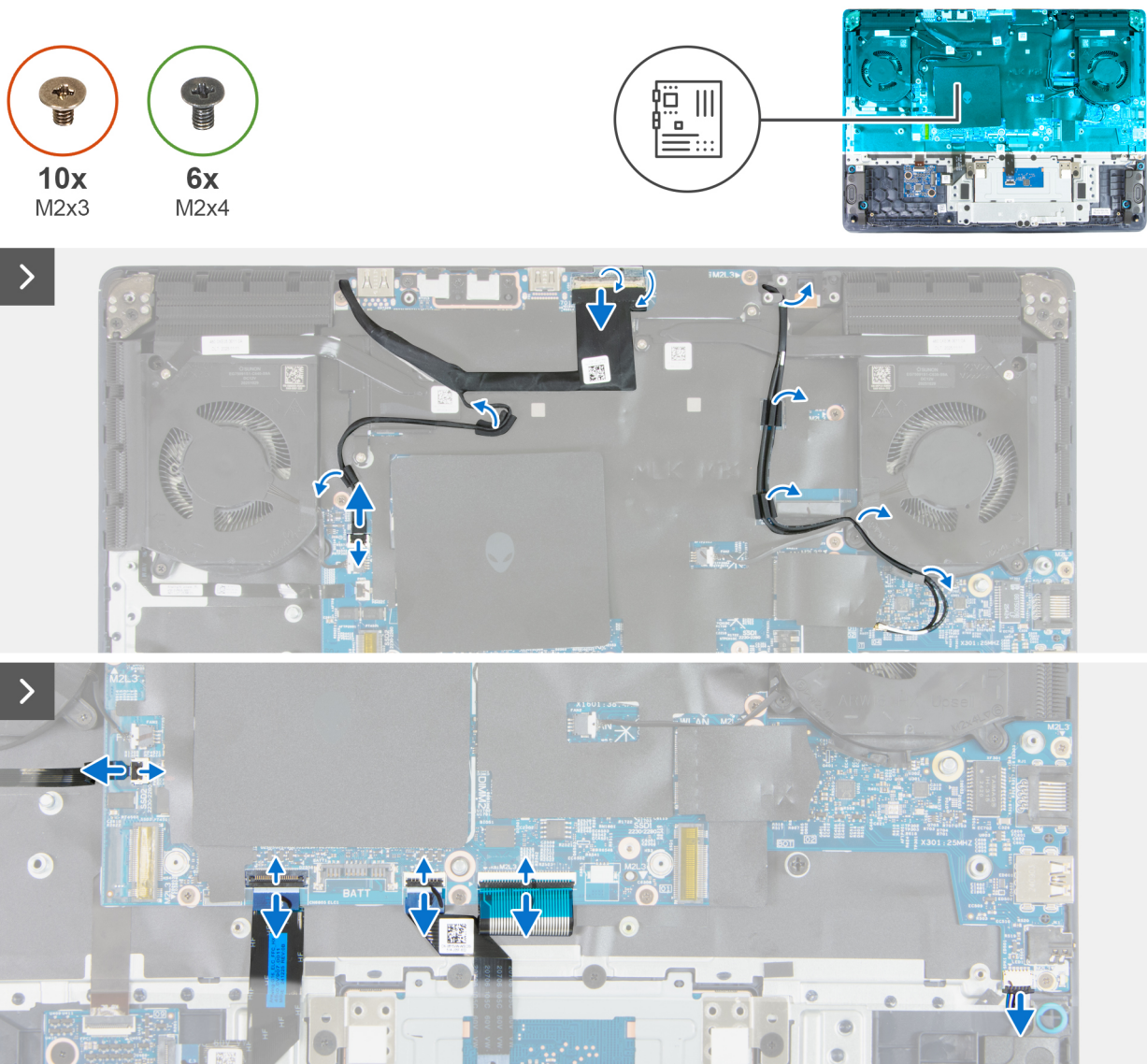
Figure 62. Removing the system board (for computers with VR heat sinks)
