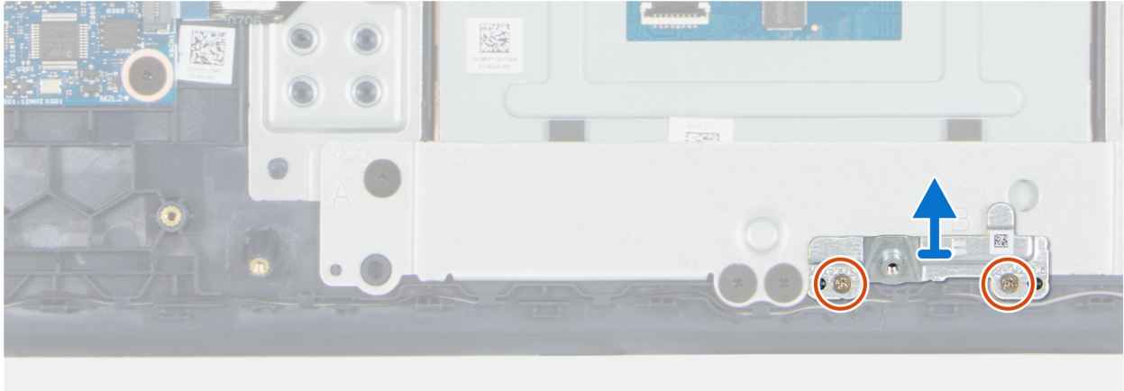
Figure 42. Removing the battery bracket
