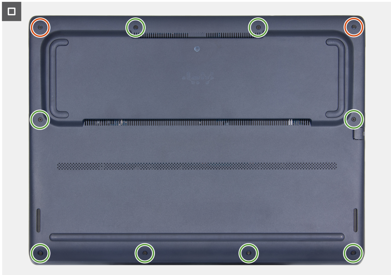
Figure 17. Installing the base cover
