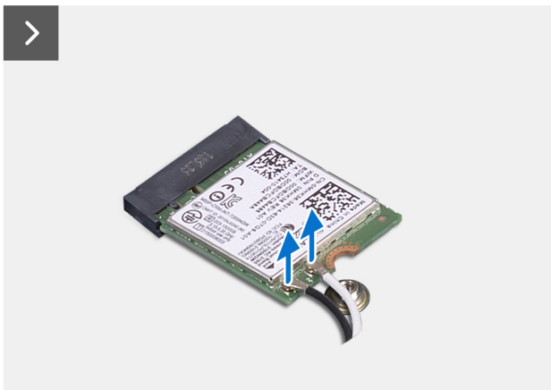
Figure 34. Removing the wireless card
