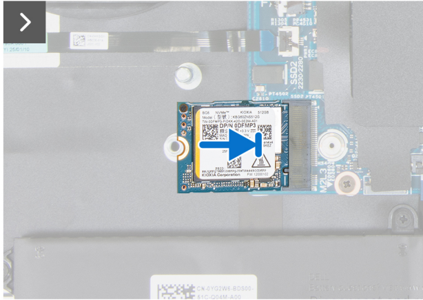
Figure 27. Installing the M.2 2230 SSD in the SSD2 slot
