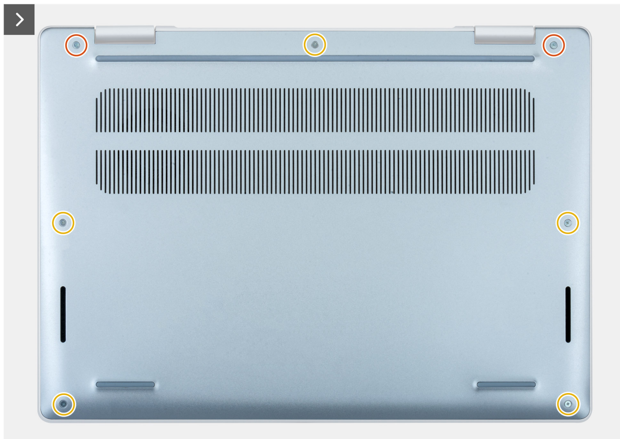
Figure 14. Loosen the screws
