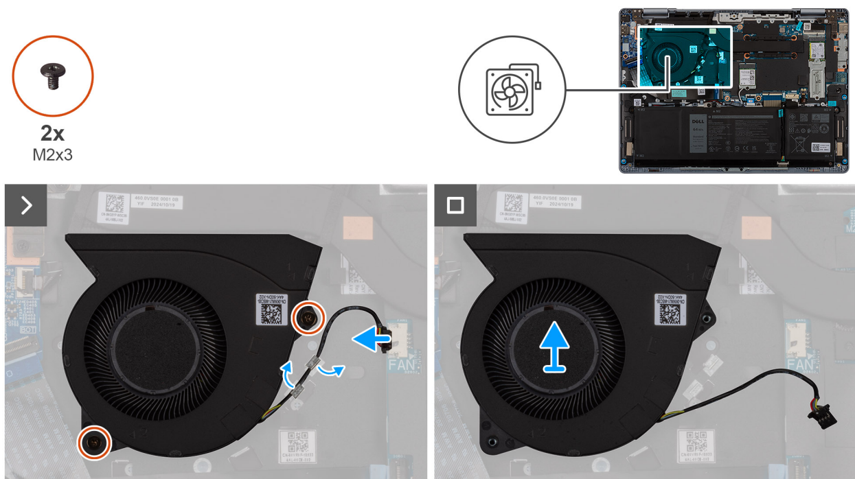
Figure 26. Removing the system fan
