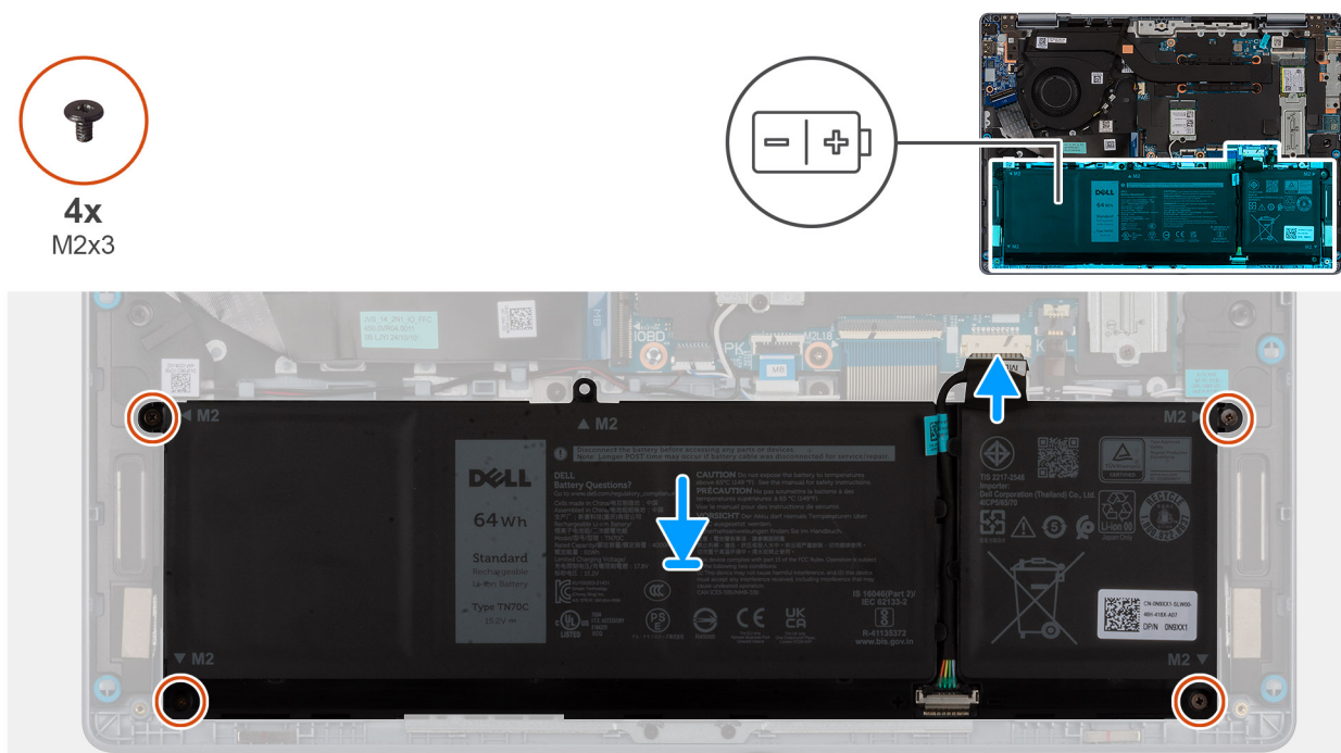
Figure 19. Installing the battery
