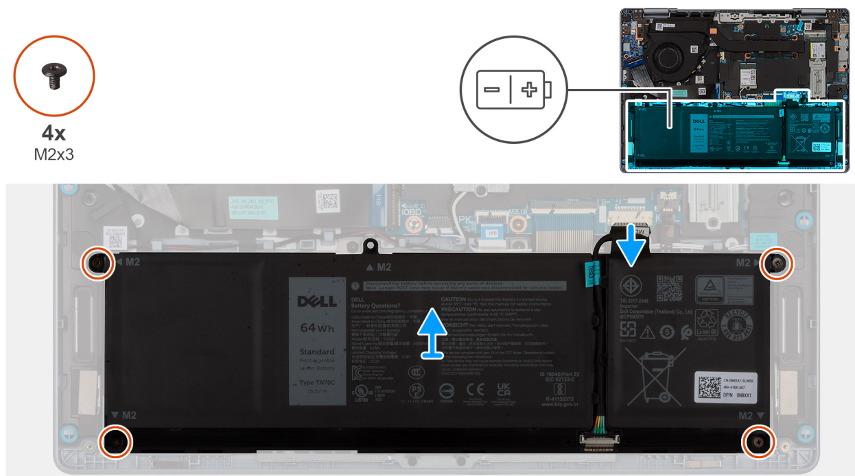
Figure 18. Removing the battery
