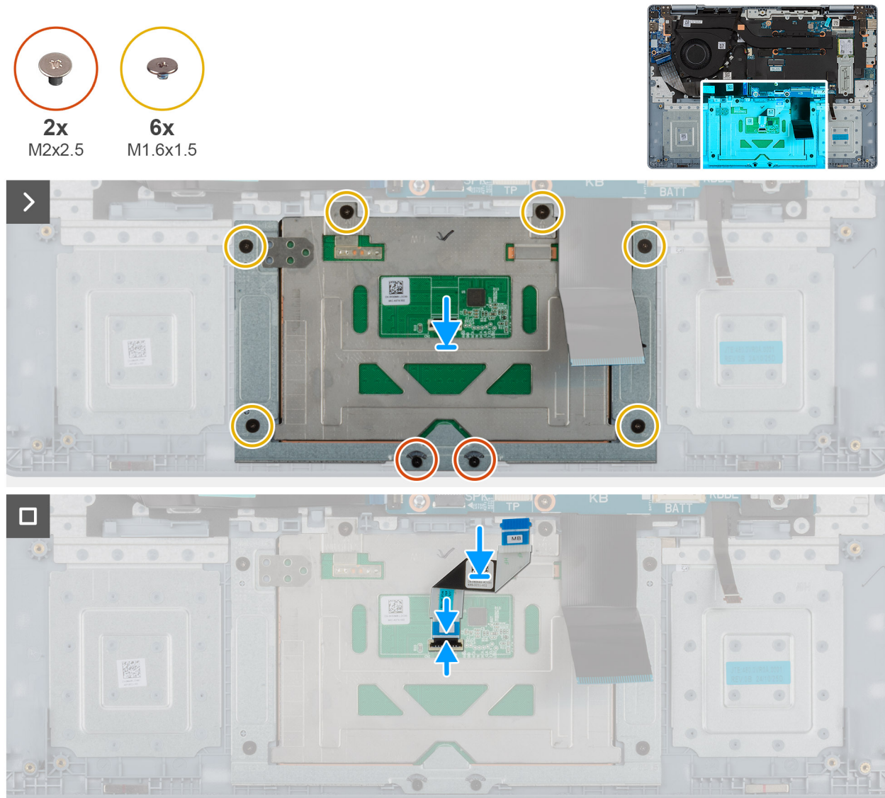
Figure 37. Installing the touchpad
