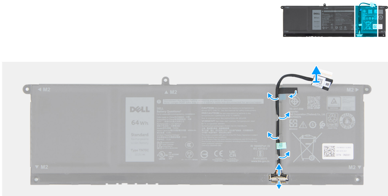
Figure 20. Disconnecting the battery cable
