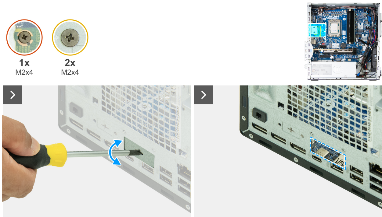
Figure 82. Installing the fiber-optic port module
