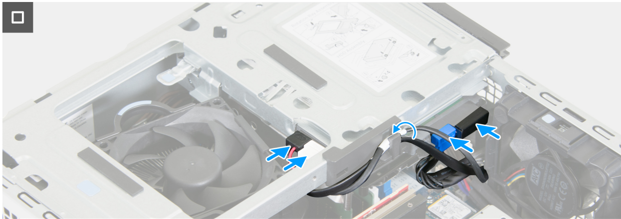
Figure 52. Installing the drive bay
