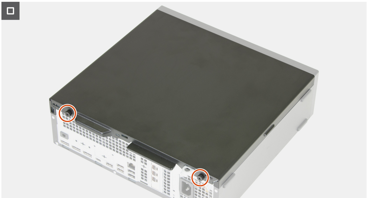
Figure 9. Installing the side cover
