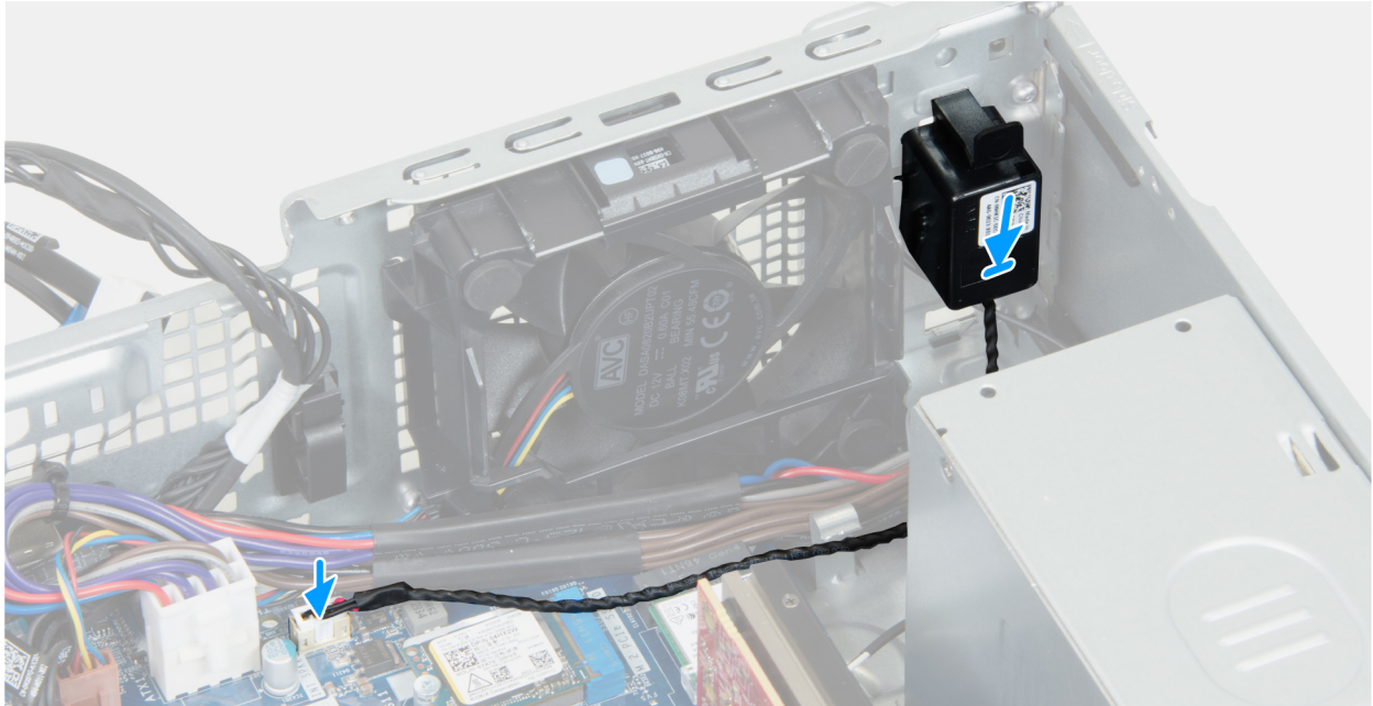
Figure 19. Installing the internal speaker
