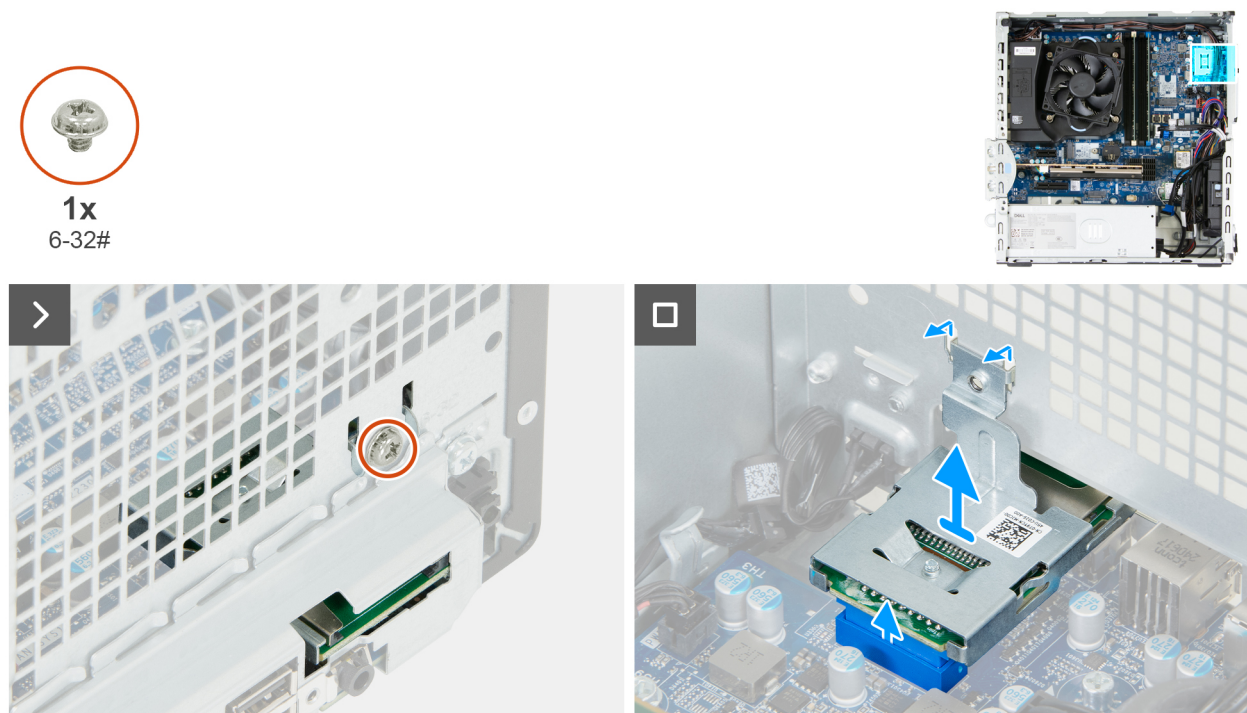
Figure 66. Removing the media-card reader
