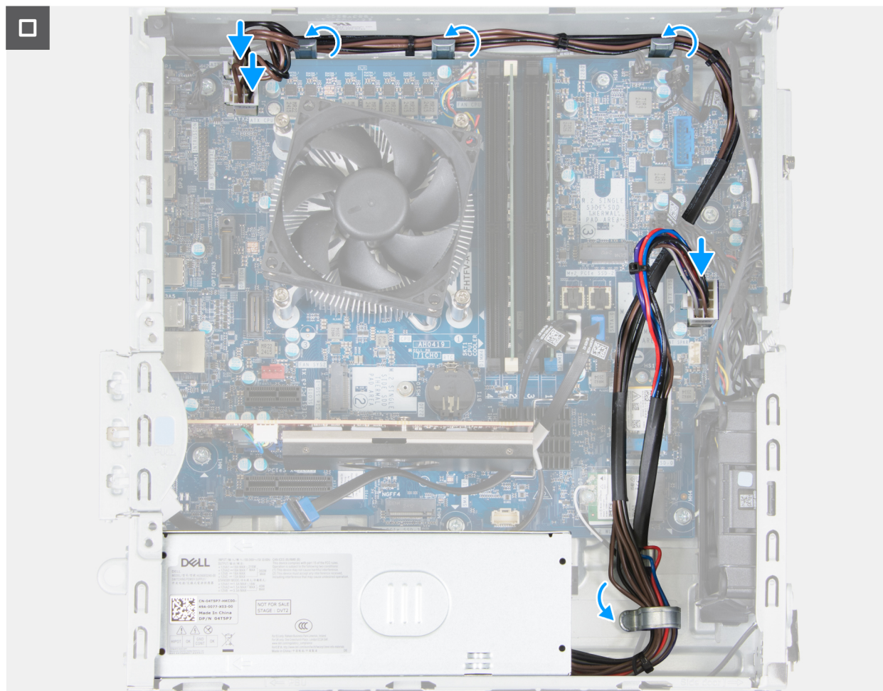
Figure 73. Installing the power-supply unit
