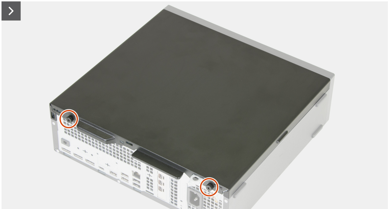
Figure 6. Removing the side cover
