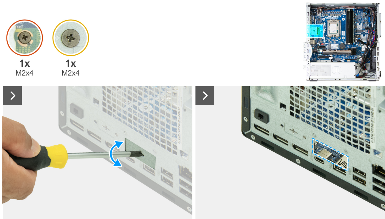
Figure 79. Installing the optional-port module
