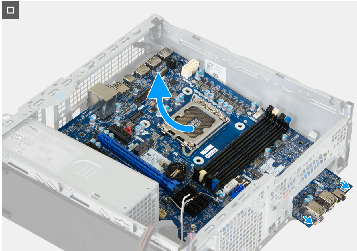
Figure 90. Removing the system board
