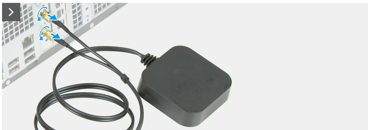
Figure 41. Removing the puck-antenna expansion card
