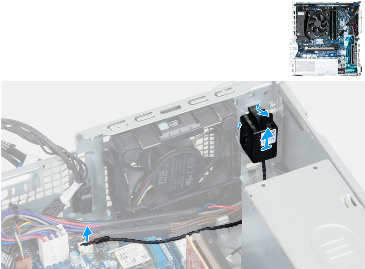
Figure 18. Removing the internal speaker
