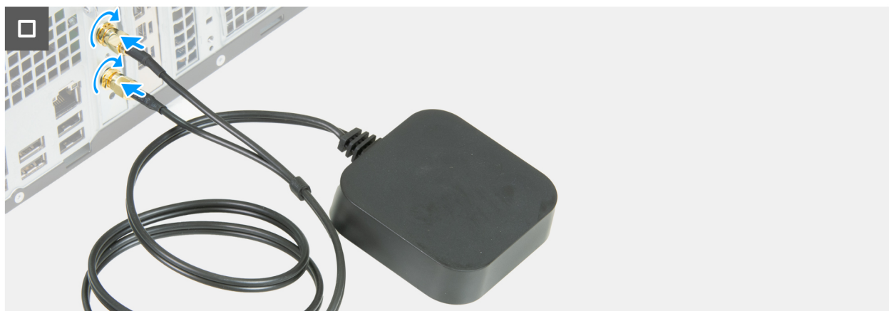
Figure 44. Installing the puck-antenna expansion card
