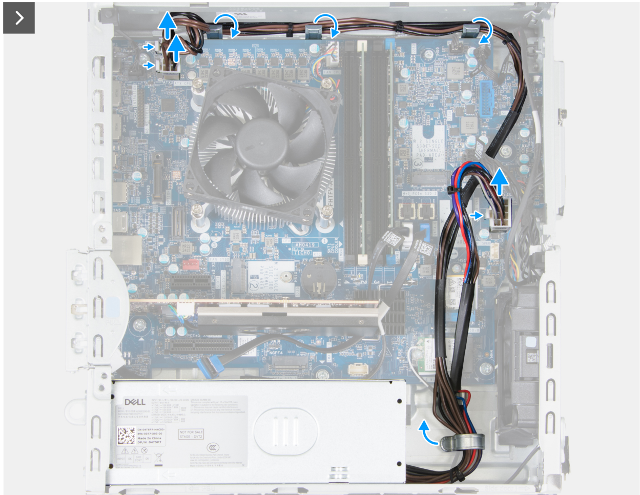
Figure 70. Installing the power-supply unit
